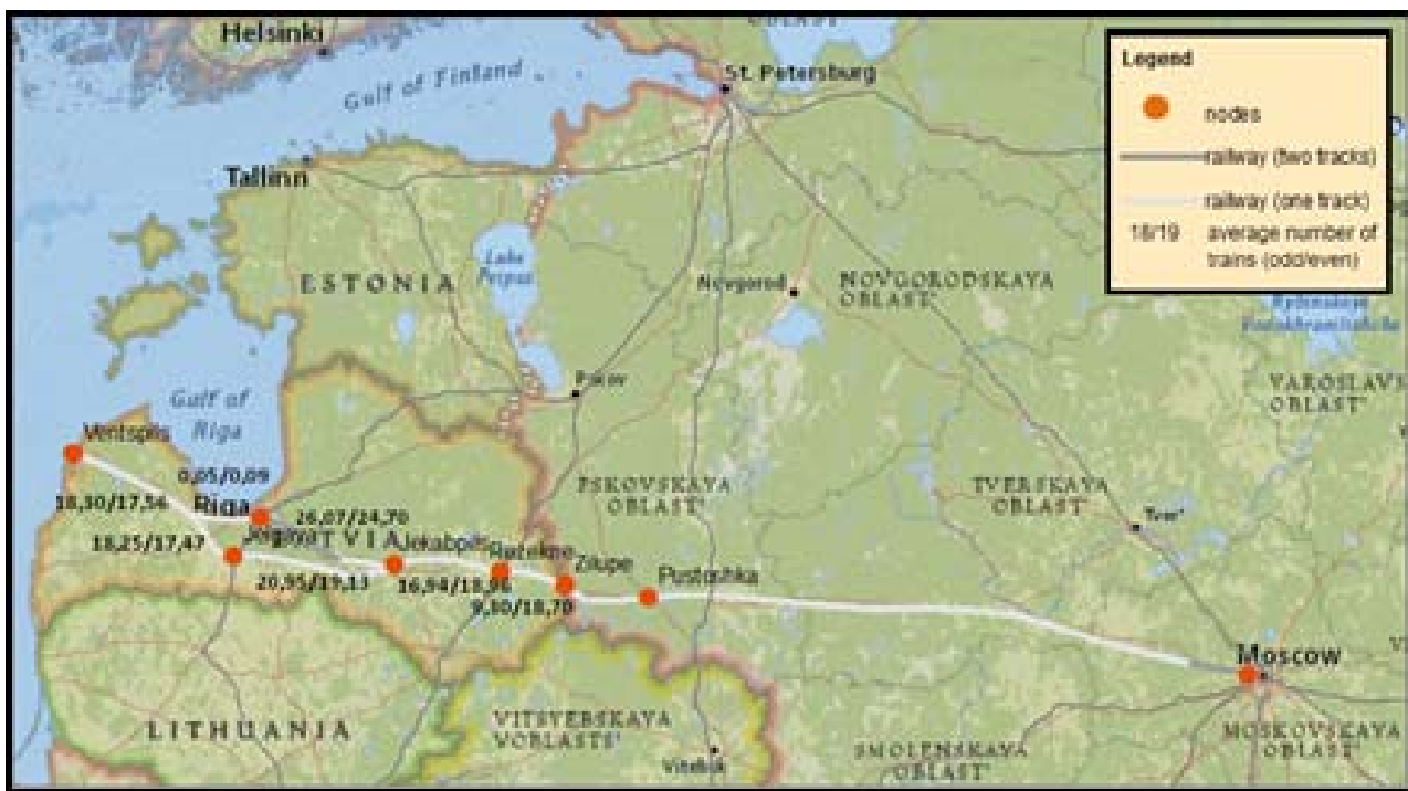
Figure 5: Level of daily traffic in 2012 (average annual number of trains), Source: Network Assessment 2013 of Latvian Railways, http://www.ldz.lv/texts_files/2013_Tikla_Parskats_EN.pdf
